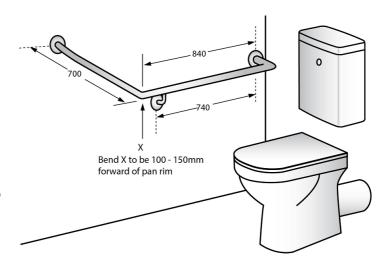
This product is AS1428.1 compliant (accessible compliant) when installed in accordance with the guidelines.
